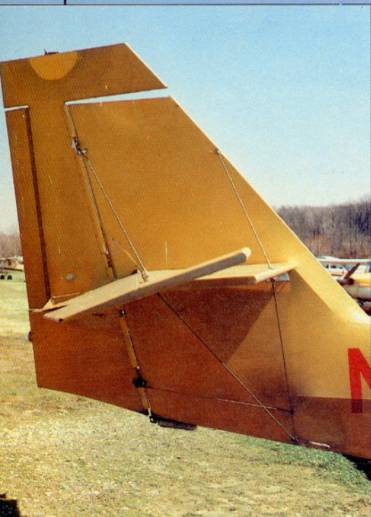
The tail section of the Lancer 402 incorporates a large rudder with an equally large rudder trim-tab. Note the profile of the horizontal stabilizer and the wire bracing. Scrub brush is situated on the underside.
