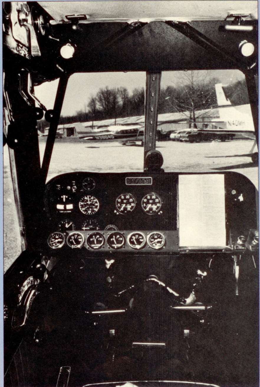
The panel is dominated by engine gauges and includes a useful checklist platform to the right. Starter cords hang from the overhead and the plane has heel, not toe, brakes.
